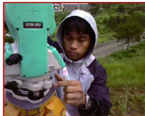
Figure 2: Setting up the Total Station for Landslide Monitoring.
